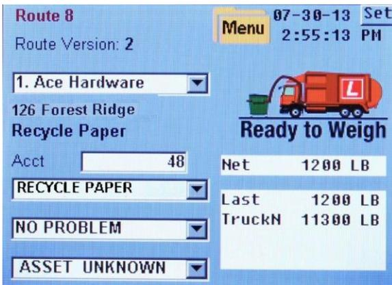
The LM400 touch screen provides all the information a driver needs to understand the status of the weighing system.
